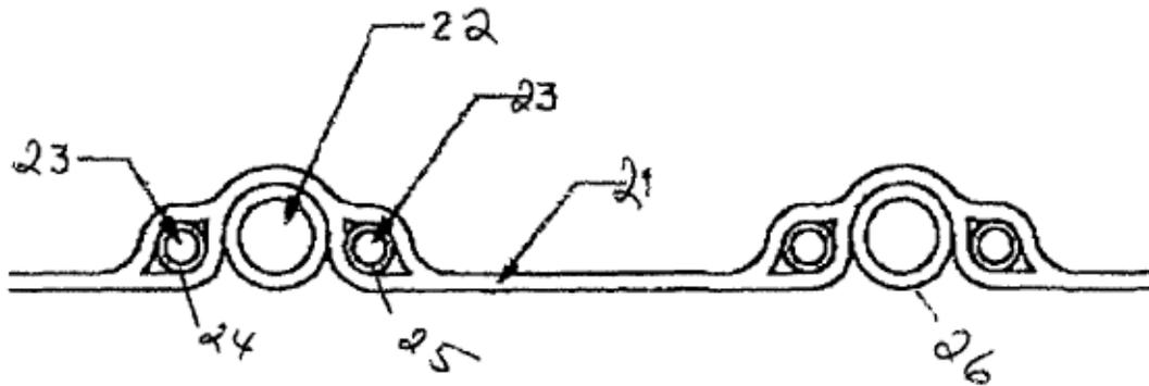
Figure 3 depicts a cut-away view of one embodiment of the hose of the '127 patent. *Id.* at 3:29–30. In this embodiment, there are insulated conductor wires 24 and 25 on opposite sides of structural helix 22. *Id.* at 4:43–47.
